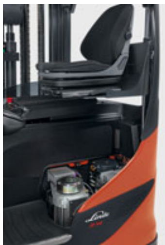
Swivel-mounted operators seat for ease of service access
