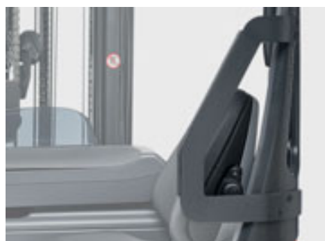
Side shoulder guard for enhanced operator protection in confined spaces
