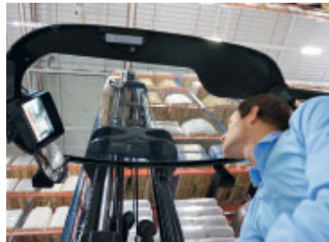
Linde panoramic High Vision armoured glass roof for unrestricted upwards visibility
